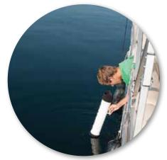
In cooperation with the UNH Cooperative Extension service, water quality samples are taken at several key spots around the lake. The team tests for water temperatures at multiple depths, measures water clarity in both sunlight and shade, takes various chemical measurements (pH, conductivity, etc.), and collects both surface and depth water samples that are sent to the UNH lab for further analysis.
